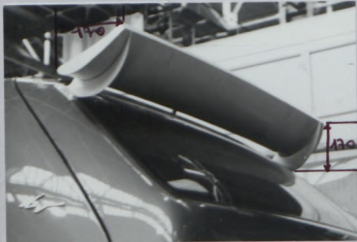
XVII) DISPOSITIF AERODYNAMIQUE ARRIERE VU DE COTE ET VU DESSUS : REAR AERODYNAMIC DEVICE SEEN FROM ABOVE AND IN SIDE VIEW:
